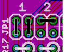
By setting jumpers on JP1 and JP2, you can select normal or bipolar operation for each CV channel. When setting two jumpers like on channel 1 of the picture above, the channel is in bipolar mode. Channel 2 in the picture is in normal mode. Please select one mode for every channel, even for channels you won't use! If you have left out the parts for the bipolar option, you can solder bridges instead of the horizontal jumpers.
