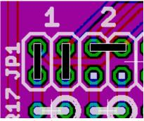
By setting jumpers on JP1 and JP2, you can select normal or bipolar operation for each CV channel. When setting two jumpers like on channel 1 of the picture above, the channel is in bipolar mode. Channel 2 in the picture is in normal mode. Please select one mode for every channel, even for channels you won't use! If you have left out the parts for the bipolar option, you can solder bridges instead of the horizontal jumpers.
