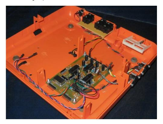
As the keypad descends towards the front, I laid all larger parts (mainly the electrolytics) flat on the boards. The clearance between the boards is quite narrow but sufficient not to fear any shorts etc.
