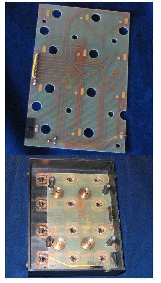
There's some space under the keypad, so I decided to mount the Core directly onto the backside of the keypad - the OPL3 module will still fit beneath it.
