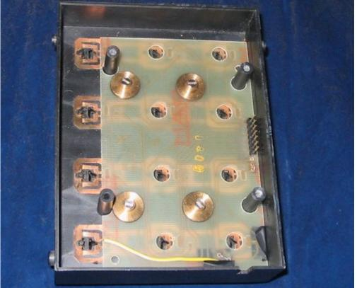
There's some space under the keypad, so I decided to mount the Core directly onto the backside of the keypad - the OPL3 module will still fit beneath it.
