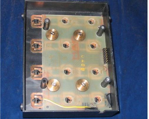
There's some space under the keypad, so I decided to mount the Core directly onto the backside of the keypad - the OPL3 module will still fit beneath it.
