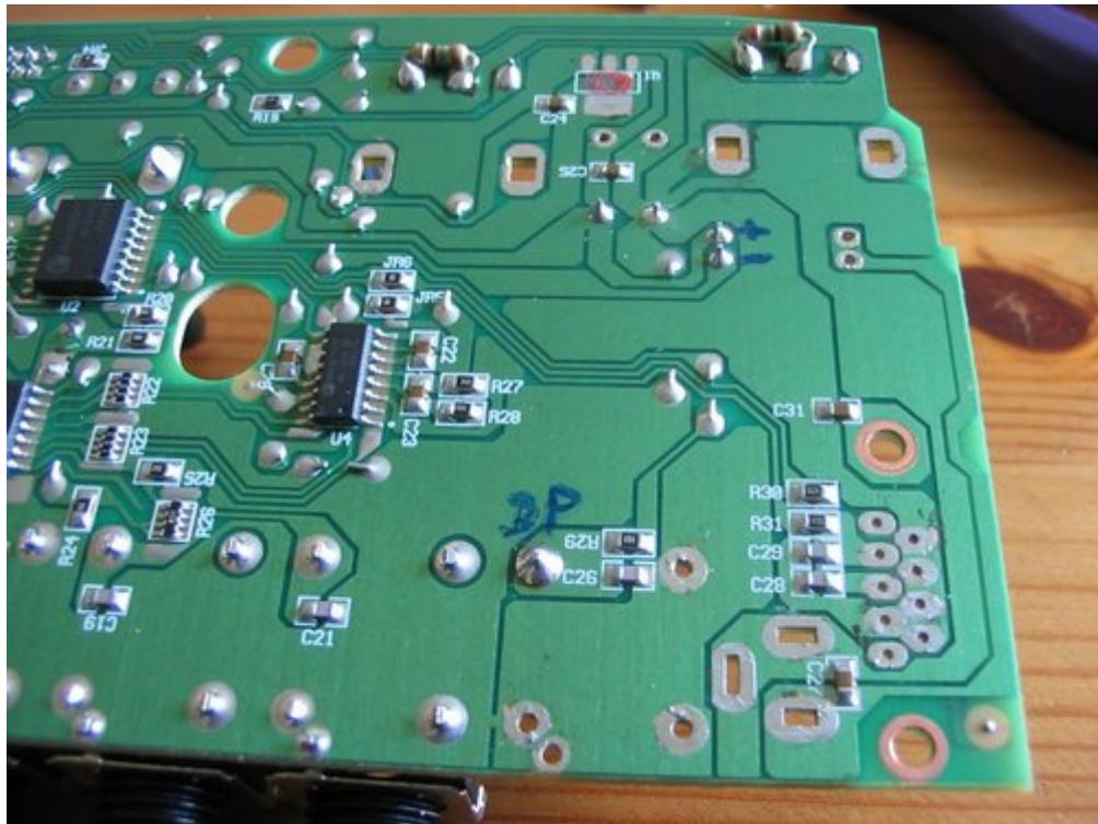
This is the lower board mounted and connected to the audio in/out jacks. Again, the capacitors are laid flat.
