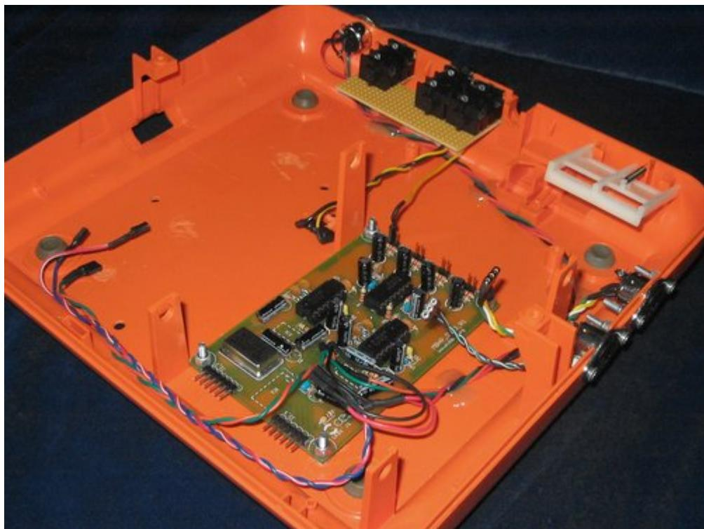
As the keypad descends towards the front, I laid all larger parts (mainly the electrolytics) flat on the boards. The clearance between the boards is quite narrow but sufficient not to fear any shorts etc.
