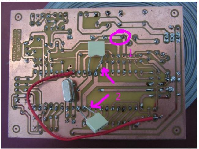
3: this seems to be a bad ground connection directly at the 78xx - it can lead to the wrong voltage. Here the same: just solder the pads again, it will help And same like above: the long cap legs need to be cutted, the danger for shorts is too high!
