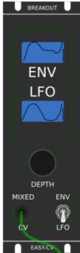
**Envelope Scope:** show the ENV-Waveform or the Mixed-CV-Output-Waveform (when Switch is in LFO Mode) and show the Envelope-Amount with a BAR
