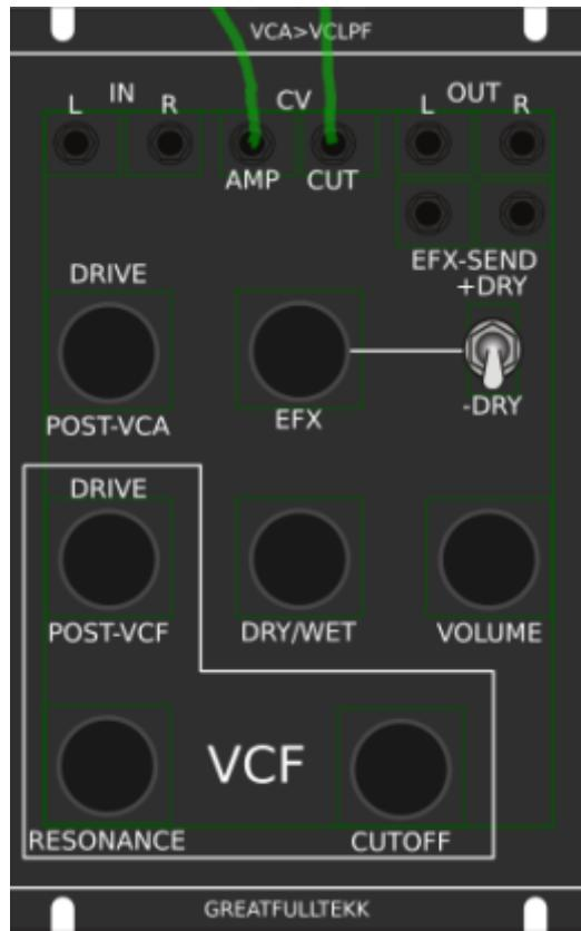
basically a simple VCA (MS20Like) that drives the input of a Audio transformator 1:3 which is a Neutrik NTE10-3 (9€)
