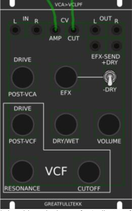
basicly a simple VCA (MS20Like) that drives the input of a Audio transformator 1:3 which is a Neutrik NTE10-3 ( $9 \in$ )
