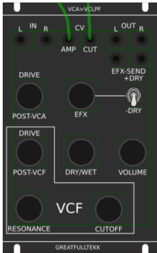
basicly a simple VCA (MS20Like) that drives the input of a Audio transformator 1:3 which is a Neutrik NTE10-3 (9€)
