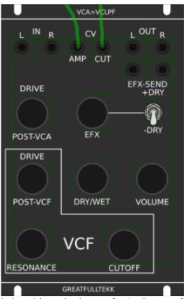
basicly a simple VCA (MS20Like) that drives the input of a Audio transformator 1:3 which is a Neutrik NTE10-3 ( $9 \in$ )
