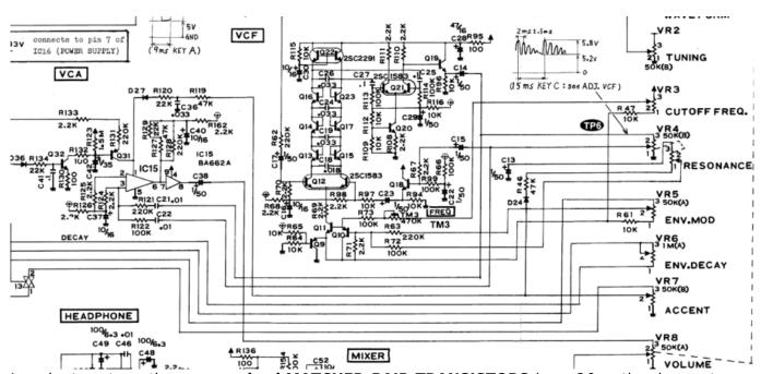
In order to not use those **overprized MATCHED-PAIR-TRANSISTORS** (over 2€ on the cheapest place) i have to use standart Transistors and make a **VBE-MATCH** on my own, i have already a PCB from here - to measure the transistors with a Multimeter: https://midisizer.com/other/vbe-matching/
