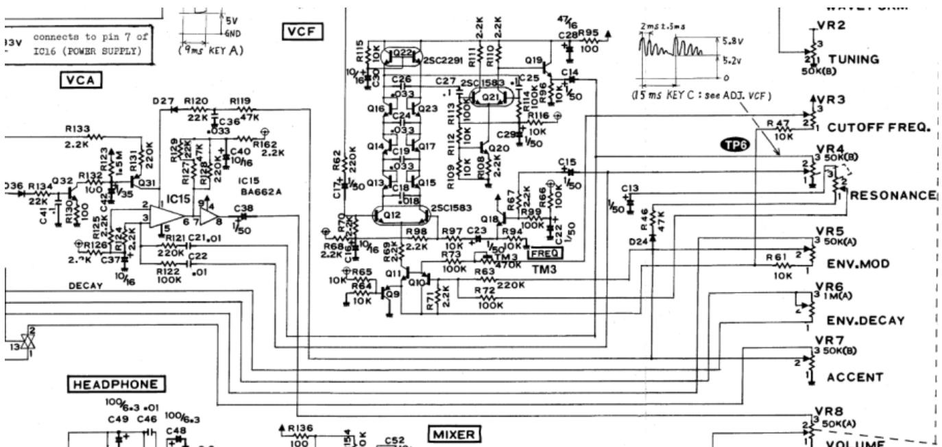
In order to not use those **overprized MATCHED-PAIR-TRANSISTORS** (over 2€ on the cheapest place) i have to use standart Transistors and make a **VBE-MATCH** on my own, i have already a PCB from here - to measure the transistors with a Multimeter: <https://midisizer.com/other/vbe-matching/>
