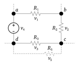
In other words, the voltage is balanced along the components rings; ad = ab + bc + cd
