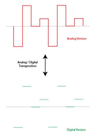
The frequency of the sampling (the little dots) is called the **sample rate**; common values are 44.1 kHz and 48 kHz. The higher the value, the better the accuracy of the digital representation.
