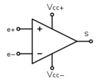
Vcc is the "power supply" voltage for the Operational amplifier
