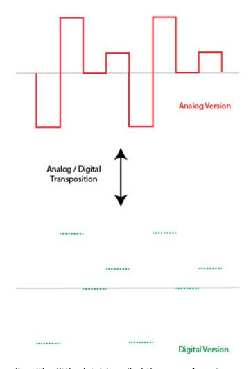
The frequency of the sampling (the little dots) is called the **sample rate**; common values are 44.1 kHz and 48 kHz. The higher the value, the better the accuracy of the digital representation.
