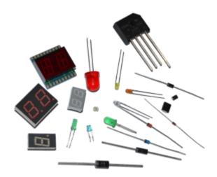
A diode is a polarized passive component that let pass the electrical flow in only one way
