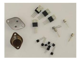
The Transistor is an **active** component that works as an **amplifier** or a **driven switch**.
