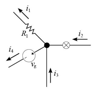
In other words, in a node, Current going to the node equals Current going from the node
