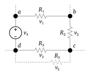
In other words, the voltage is balanced along the components rings; ad = ab + bc + cd
