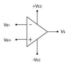
**Vcc is the Bipolar power supply voltage** for the operational amplifier . It is assumed it exists , but not always represented to make things clearer
