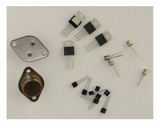
The Transistor is an **active** component that works as an **amplifier** or a **driven switch**. **BJT**s and **FET**s perform **similar** functions, but with a **different type of input**. Both kinds of transistors are devices that control the current flowing through them and can be used as digital switches or analog amplifiers.
