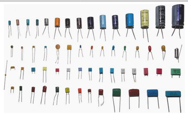
The capacitor is a **passive** component used to store electrical energy temporarily in an electric field with a value in **farads**. It is sometimes Polarized (Electrolytic, like the top line of capacitors in the picture above), sometimes not (Ceramic, like the 3 bottom lines of the picture above)
