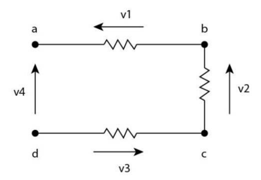
In other words, the voltage is balanced along the components rings; ad = ab + bc + cd
