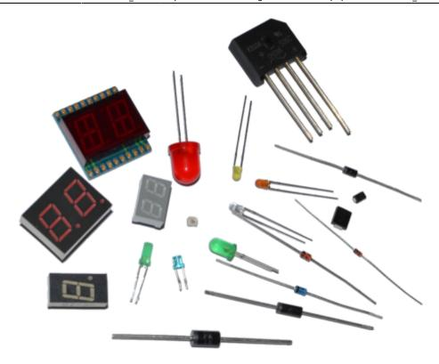
A diode is a **polarized passive** component that let pass the electrical flow in only one way . It acts like an anti-return system for electricity. By building a quad diode bridge you can make a voltage rectifier. It can also produce light (ex : LED)
