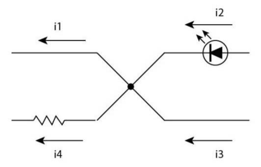
In other words , in a node , Current going to the node equals Current going from the node
