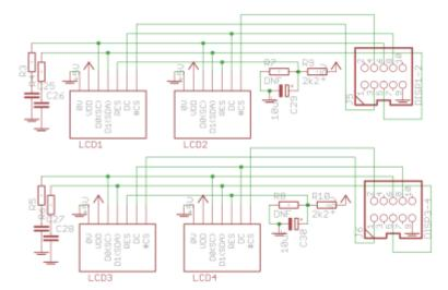
The reset circuits R9/R10/C29/C30 should be installed. The termination circuits R3-6/C25-28 shouldn't be required. When wiring ribbon cables, the end attached to the ELO board should have two IDCs on it; there is no connection on the PCB for the clock/data etc. lines between the two pairs of displays.
