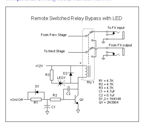
"The neat way to defeat the clicks is to slow down the change in voltage across the inductor. The circuit at left does that. An
