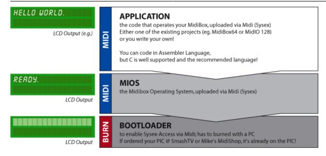
MIOS is the operating system of the Microchip PIC18F\* chip, in a Core module. It can be uploaded by SysEx (via MIDI) thanks to a bootstrap loader, a special software that is already burned onto the chip if you order at SmashTV's or Mike's Shop.
