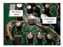
Here the signals are centered around 2.5 volts. After a few experiments I found that these signals are too weak to be fed directly into the LPCXpresso board's ADC inputs, they need some gain. The output signal of the force sensor is captured too, of course the timing requirements are much less demanding here. Here the voltage is taken directly from the force sensing resistor, just via a simple RC low pass filter to suppress noise.
