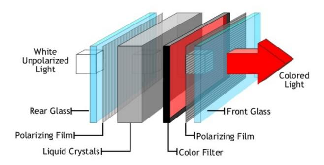
Monochrome LCD images usually appear as blue or dark gray images on top of a grayish-white background. Color LCD displays use two basic techniques for producing color, passive matrix is the less expensive of the two technologies.
