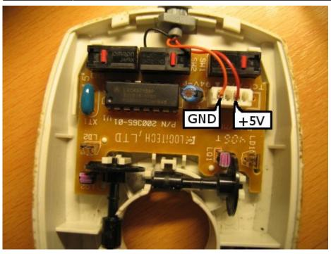
I have removed the other two cables from the connector to use them for the signals of the phototransistors.
