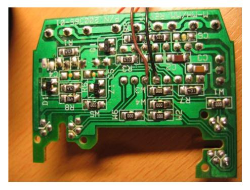
On the DIN board, you'll need to remove the pull-ups resistors, because the phototransistors signals cables already output a stable voltage (either 0V or approx. 5V). I haven't tested with the pull-ups resistors on, but I think it won't work, because the mouse PCB works with very low currents.
