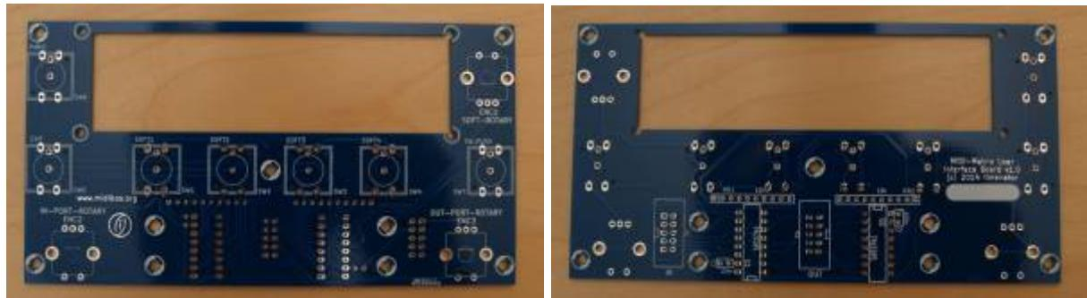
The total size of the PCB is 150mm x 80mm.
