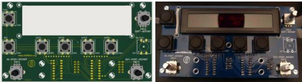
A second generation PCB as pictured above has been ordered and tested to work. This PCB can also be used with other projects involving an SCS, e.g. the [MIDIbox NG](#). Both, my favourite switches from [Marquardt \(6425 series\)](#), as well as the [E-Switch TL1100 series](#) (see e.g. MB SEQv4) can be used.
