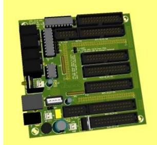
On the left is a rendering of the FPGA board created with KiCAD. This is the second generation v1.1 FPGA board which has a pair of MIDI I/Os, and an AC power plug (which can also be used to feed DC power). The board can loop through the USB signals from the Micro USB plug found on the STM32F4 Discovery board to the outside world when the whole unit is mounted in an enclosure. The FPGA board connects to J8/J9 of the core board for DIN and DOUT chains, and to J11E for MIDI connectivity.
