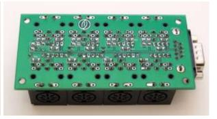
Because I like the idea of recycling components that have barely been used in other, now obsolete equipment, the MIDI sockets can also be replaced with DIN sockets bearing different kinds of footprints and/or additional pins. I frequently use 8-pin DIN sockets de-soldered from old video equipment as they are fully compatible with the 5-pin MIDI plugs. Of course, the standard 5-pin MIDI socket footprint will fit here as well!
