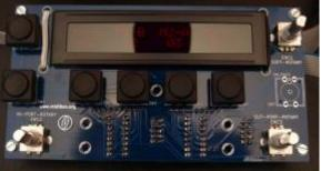
A second generation PCB as pictured above has been ordered and tested to work. This PCB can also be used with other projects involving an SCS, e.g. the MIDIbox NG. Both, my favourite switches from Marquardt (6425 series), as well as the E-Switch TL1100 series (see e.g. MB SEQv4) can be used.
