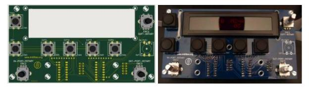
A second generation PCB as pictured above has been ordered and tested to work. This PCB can also be used with other projects involving an SCS, e.g. the MIDIbox NG. Both, my favourite switches from Marquardt (6425 series), as well as the E-Switch TL1100 series (see e.g. MB SEQv4) can be used.
