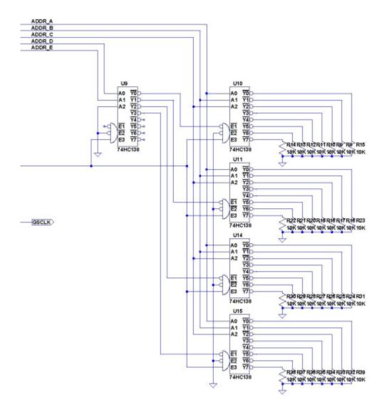
ADDR\_x, ADDR\_CLK, GSCLK are connected to the top board...
