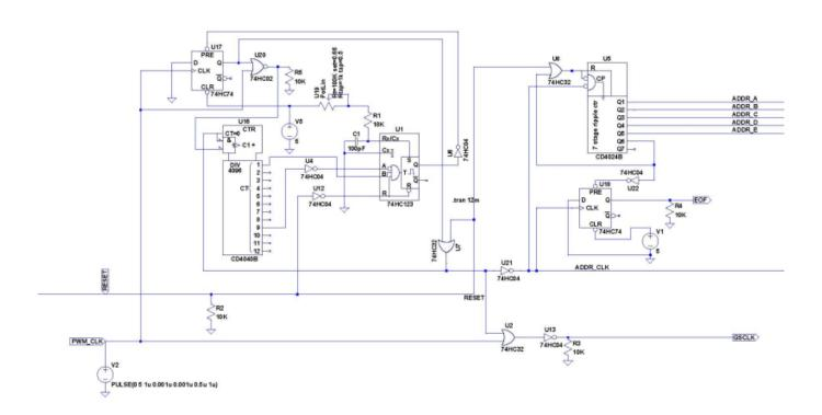
The external clock circuit was simulated on LTSpice first and tested on veroboard with the prototyped OLRE16.
