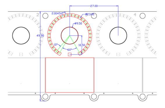
By reversing OLED displays, the active area is closer to the ring.
