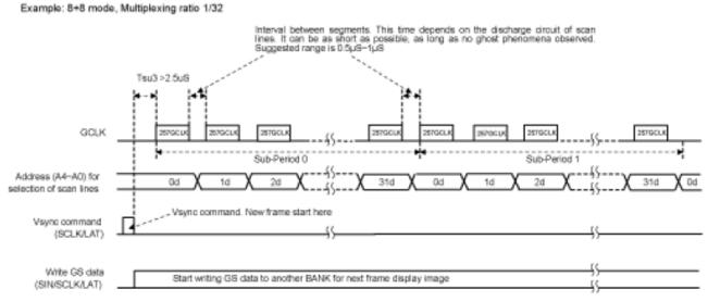
Figure 16. Controller Timing Sequence, 8+8 Mode, 32 Multiplexing
