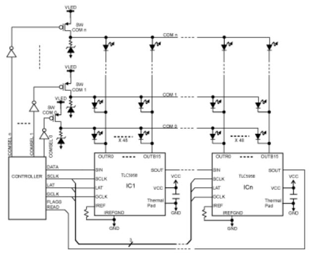
Figure 1. Typical Application Circuit (Multiple Daisy Chained TLC5958s)
