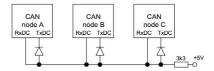
With transceivers on a 2 wire buss. All nodes are in parallel over the buss.
