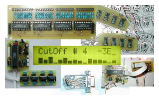
The MIDIbox Hardware Platform is the continuation of the work of Thorsten Klose on MIDI controllers in the past several years. It brings every MIDI controller design down to one standardised environment with reusable and exchangeable modules. Modular construction is nothing new in electronic devices.
