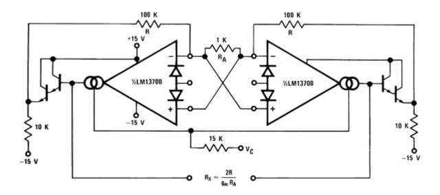
A floating VCR where each "end" of the "resistor" may be at any voltage within the output voltage range of the LM13700.
