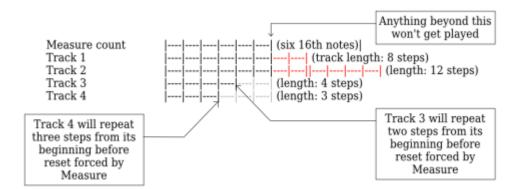
It's also possible to sync tracks to measure manually on the MENU + MANUAL page. Pressing SELECT on this page will sync the selected tracks to measure. Tracks can be selected either with the group and track selection buttons (top left of the frontpanel) or on the Track Selection page (for details, see section 5.6.).
