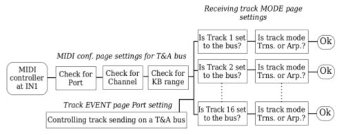
If the incoming MIDI data passes through the port, channel and keyboard range limitations, and the Jam page Fwd is set 'on', the bus that is set to the 'Jam' function will receive the incoming data and forward it to the active track's output port and MIDI channel. This is done regardless of the active track's bus settings (on the track's MODE page) (see section 6.1.1. for details on the MODE page). If
