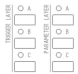
By default, trigger layer selection button A selects the gate layer, B selects accent, and C brings up a page where you can select one of the eight trigger layers with a GP button. (Drum tracks have only 1–2 trigger layers, for these see section 3.3.)
