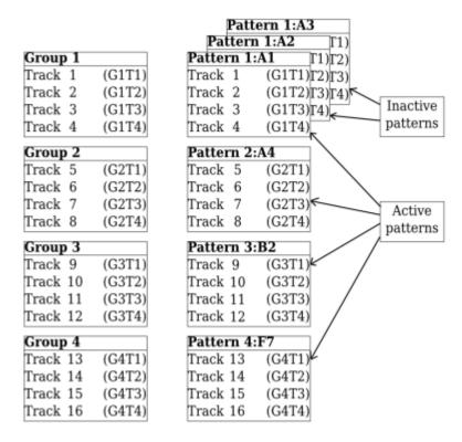
Tracks contain the data – gates, accents, notes, note velocities, CCs etc. – that you've programmed in them and that is sent over to your MIDI equipment. This data is in *trigger layers* and *parameter layers*. (For details, see section 3.)
