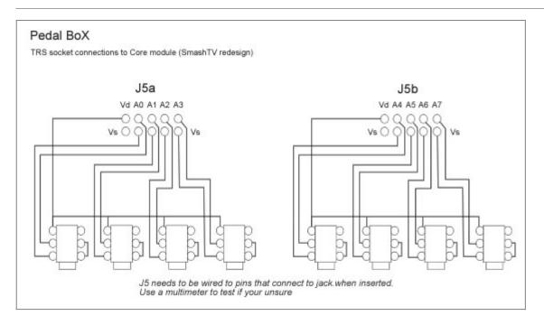
When inserting/removing a jack, make sure the control voltage = 0 (pedal off). Or you will pass voltage straight to ground, causing mios to crash, and maybe cause damage to the circuit.
