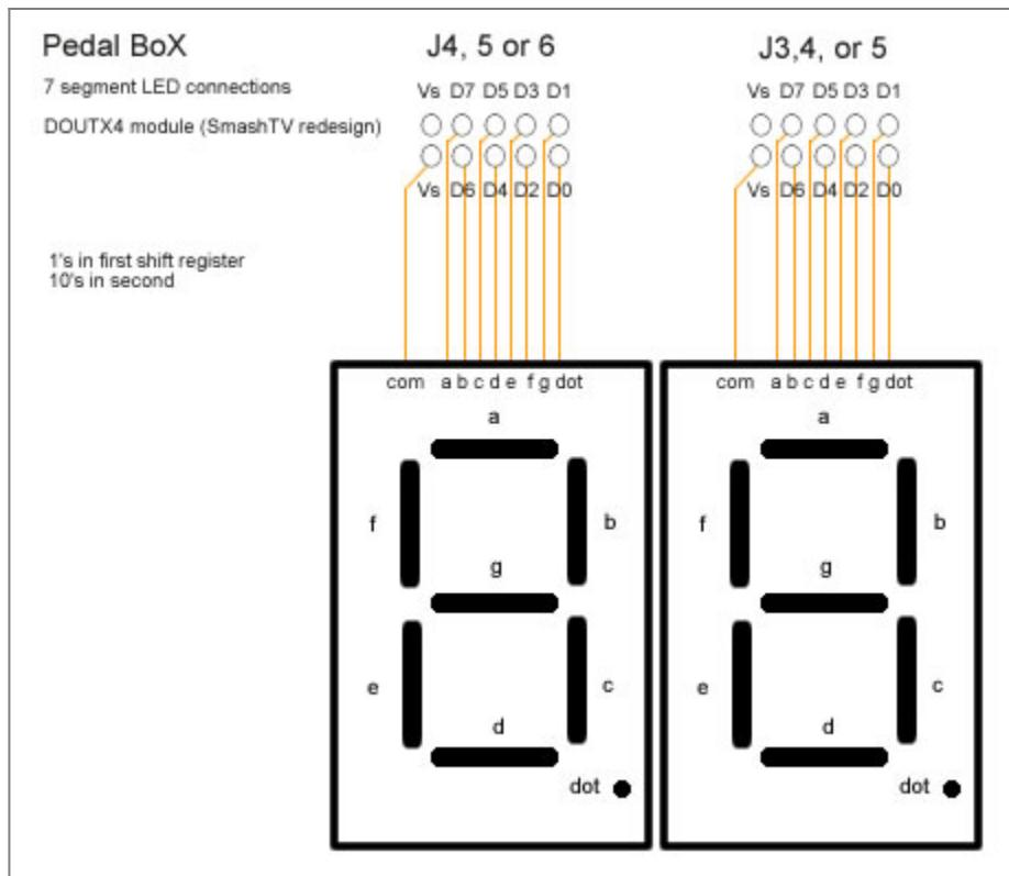
0, 1 or 2 digits can be used (defined in pbx\_config.h). If no digits are used, the current bank is displayed on the LCD (requires a 2x20 display)
