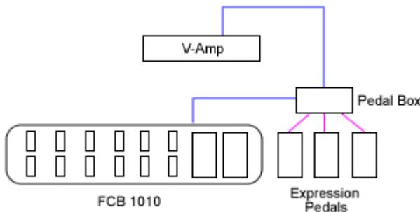
Pedal Box expands your existing floorboard with functionality very similar to Pedal Board
