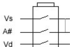
Switches connect when no jack is inserted.
