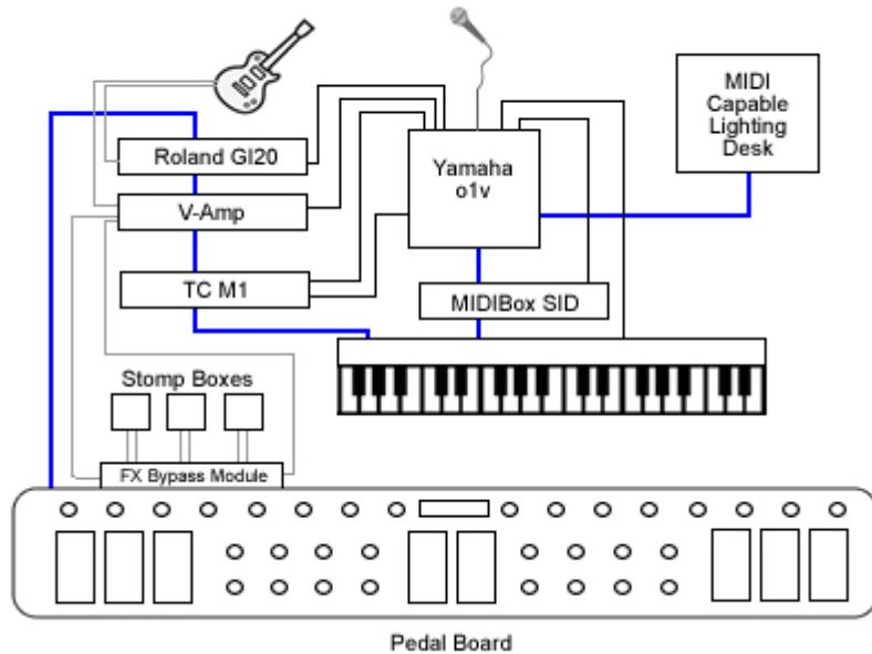
Pedal Board (and Pedal Box) can be taken to the extreme. Controlling up to 7 MIDI devices. Utilising Rig Control it can set them all to your desired settings with a single stomp.
