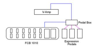
Pedal Box expands your existing floorboard with functionality very similar to Pedal Board Up to 8 Expression pedals and 8 relays can be used. Your floorboard provides the buttons.
