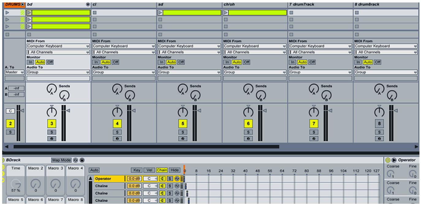
Each send/return contains an FX rack with 2 chains corresponding with 2 set of effects.
