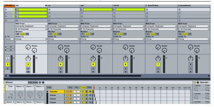
Each send/return contains an FX rack with 2 chains corresponding with 2 set of effects.
