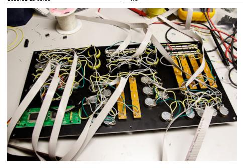
This shot shows all of the panel components wired and ready to attach to the modules.
