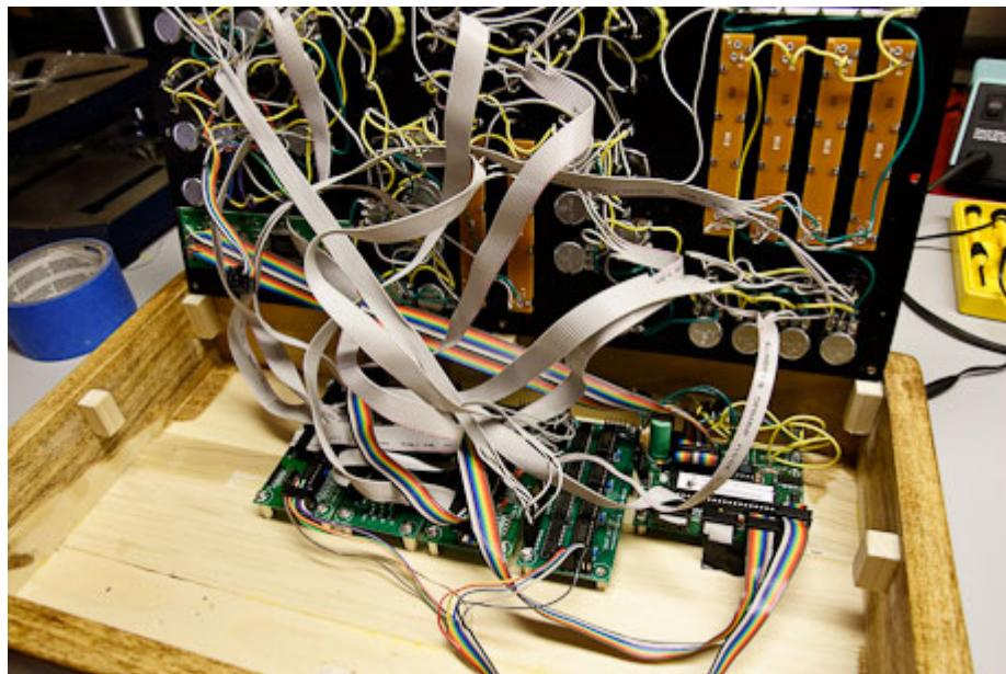
**Wiring the Panel:** Now comes the tedious and time consuming part of the build, wiring the front panel. For the most part, the PDF diagrams on the ucapps site that accompany each module are the keys to understanding the wiring sequence. I'm using ribbon cable, as it will be easy to attach to the modules, and keeps the overall spaghetti-ness of the panel down considerably.
