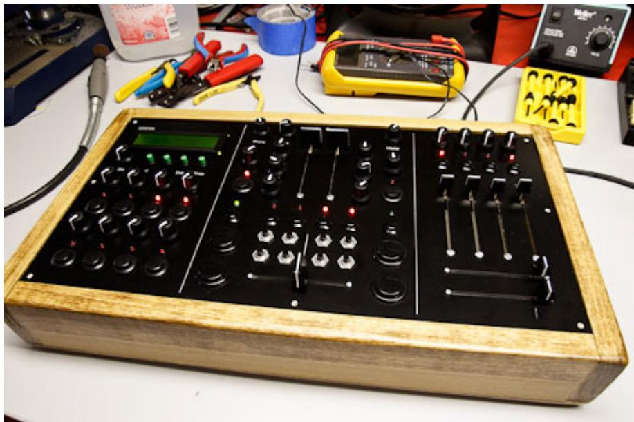
My controller is designed to provide controls for the features I use most in Traktor. Because of this, I've left out controls for features that other users might find essential (looping, pitch control, etc). There is also a section of the controller that is specifically for functions in VDMX, and will not be used for Traktor. In addition to the Midibox controller, VDMX is controlled by a DIY Arduinome (Monome <http://monome.org/> clone).
