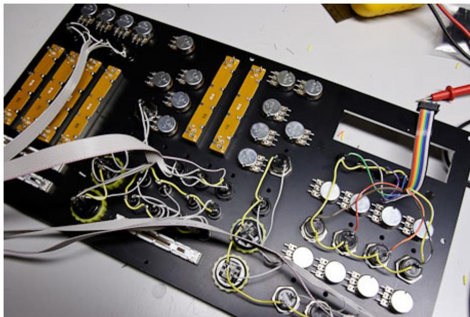
The shot above shows the DIN (pushbutton) wiring completed. I've left the ribbon cabling long until I can determine how long the runs will need to be to get to the modules.
