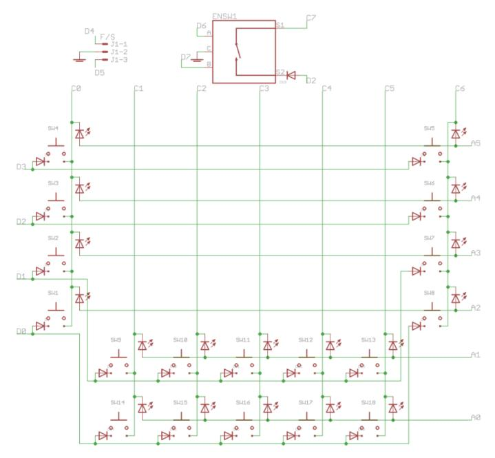
Note the encoder connected to pins D7 and D6, and header J1 connected directly to D5 and D4. All of the cathode rows are used, even C7 just for the encoder push switch.
