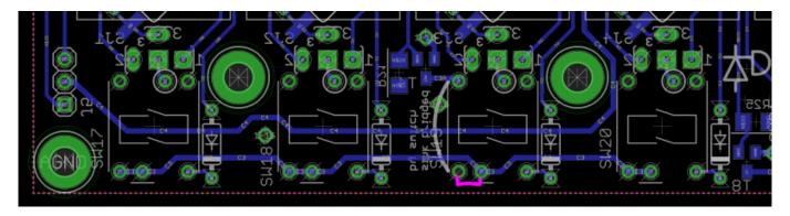
Ghosting. As seems common with these kinds of matrices, there is some unwanted lighting of LEDs. This is most apparent when trying to light up the bottom row of MEC switch LEDs, as the resistive path to the Superflux LED is lower and thus glows unintentionally. This can be overcome somewhat by
