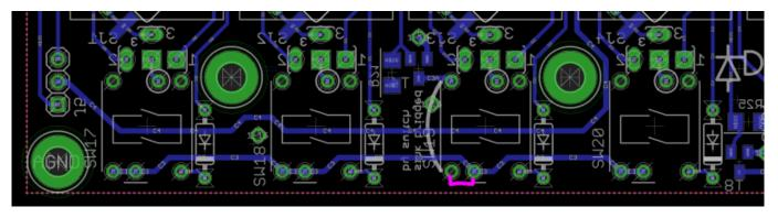
Ghosting. As seems common with these kinds of matrices, there is some unwanted lighting of LEDs. This is most apparent when trying to light up the bottom row of MEC switch LEDs, as the resistive path to the Superflux LED is lower and thus glows unintentionally. This can be overcome somewhat by stacking BAT54 Schottky diodes on top of the BC818 transistors. Later revisions will have more elegant mounting.
