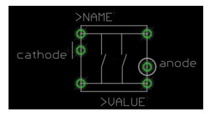
*Very important*: the Matias switches must go in <u>through the completed Plate PCB!</u> If they are put in before the Plate PCB, the **Plate PCB won't fit and there will be no way to mount the encoders!**
