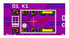
The Omron G6K-2P relay is available at several common places like Mouser, Digikey, Reichelt etc, but is a bit on the expensive side. If space is no issue, you could also use some short wires to solder in a different larger/cheaper/available 12V DPDT relay.
