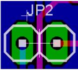
JP2, JP3, and JP4 configures the pcb to be used as a router. connect each set of pins together if you're using a router. leave them disconnected for a seq.
