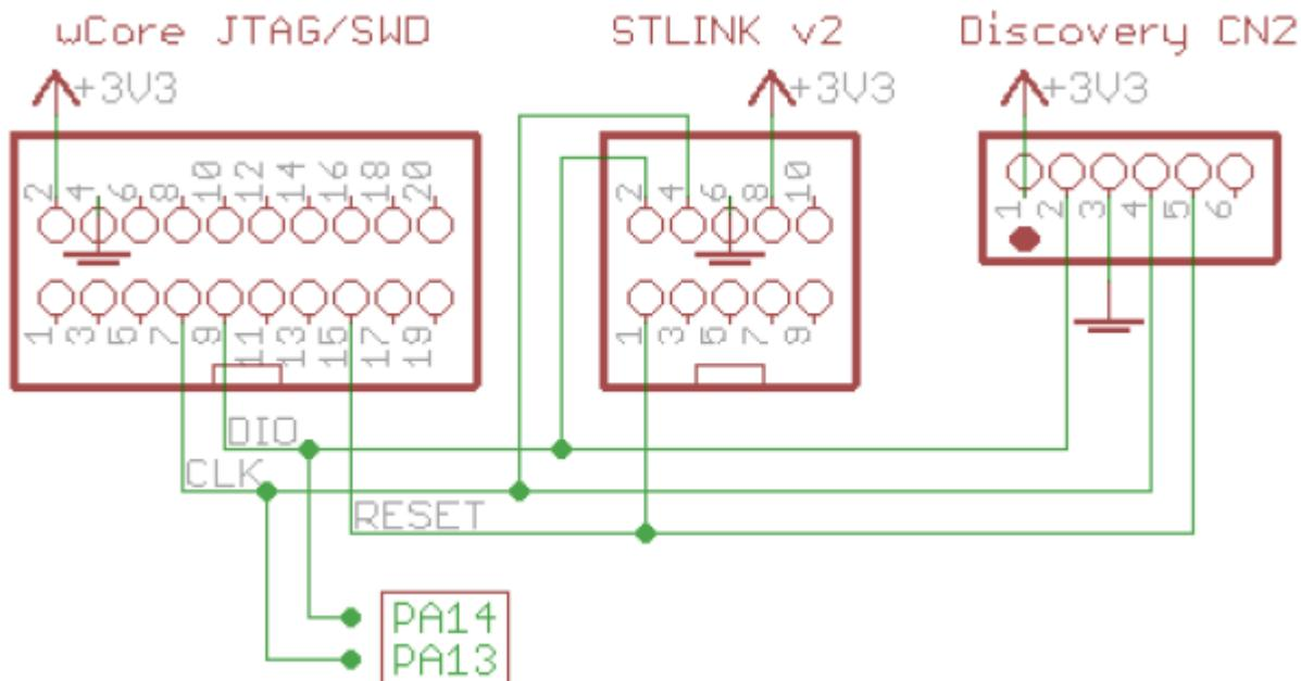
After that, [http://www.ucapps.de/mbhp\\_core\\_stm32f4.html](http://www.ucapps.de/mbhp_core_stm32f4.html) for the initial flash of a Discovery module.
